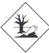
*2) If the product is not included in limited quantities and it is transported with outer packaging, UN number must be specified on the each inner label. Hazard symbols for the outer package that are mentioned above must be added with the sizes specified in the legislation. Also, orientation arrows must be used.*
